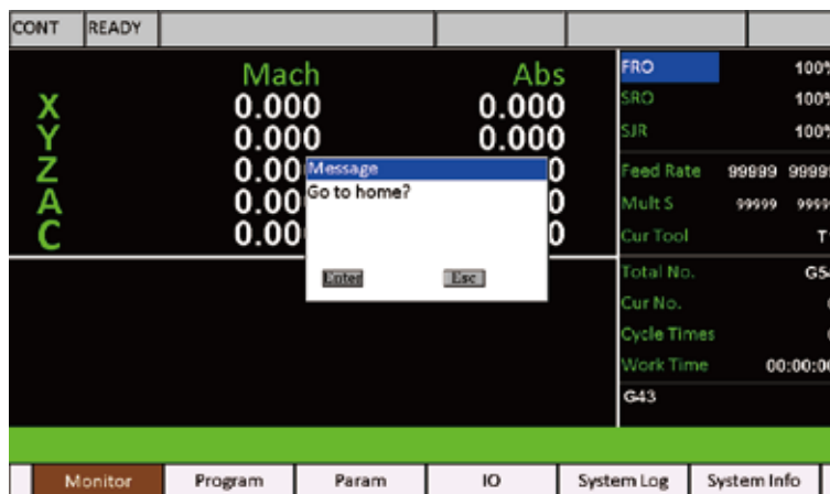
Figure 5-54 System ask If go to Home when Power on
